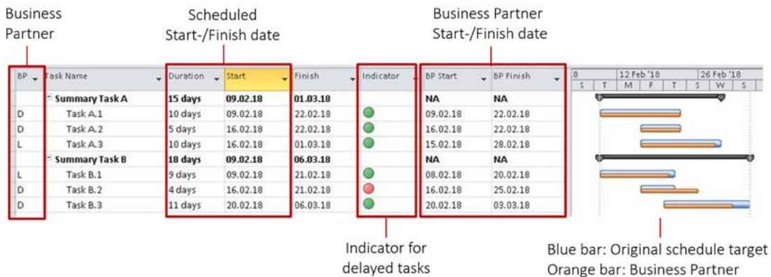
View of the data from a Primavera project in Microsoft Project shown in a table and Gantt chart
